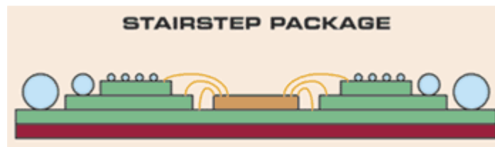
1. In this stairstep substrate design, each layer connects to the board directly.
