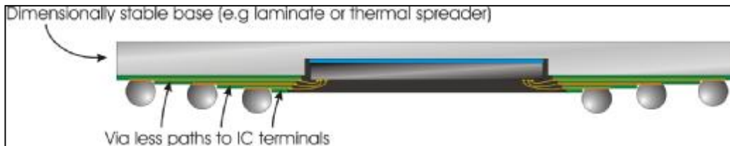
Figure 5. StairStep Package Cross-Section
